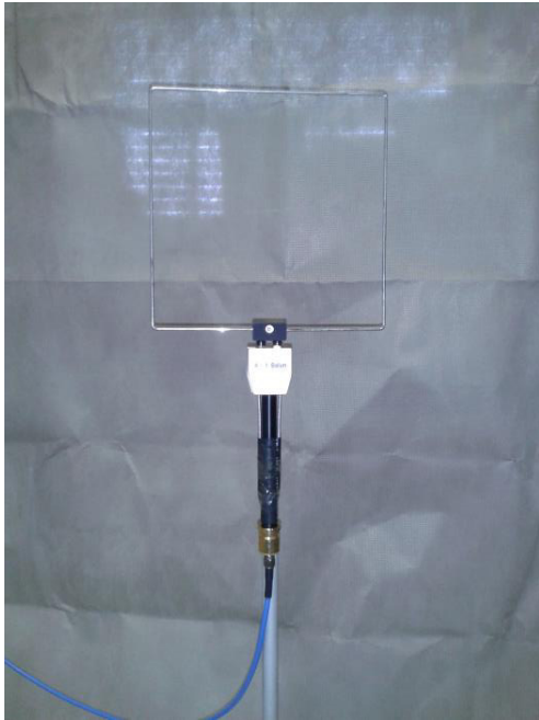
Figure 10. Quad Loop Antenna used to address the shielding effectiveness of the fabric, seen on the background.
