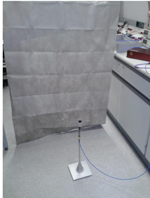
Figure 12. Two measured scenarios: (top) direct transmission and (bottom) with the conductive sheet.
